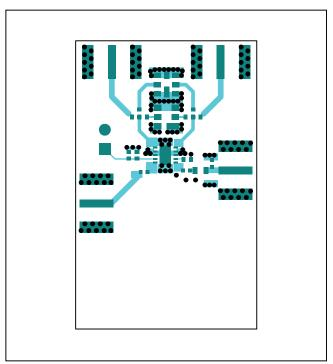
MAX2670 EV Kit Component Side—Component Side
