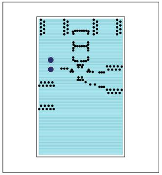
MAX2670 EV Kit PCB Layout—Layer 3 (GND)
