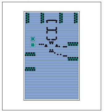
MAX2670 EV Kit PCB Layout—Solder Side
