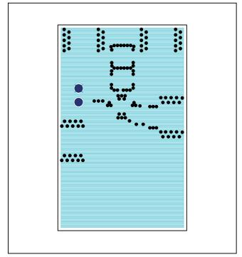
MAX2670 EV Kit PCB Layout—Layer 2 (GND)
