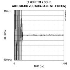
CHANNEL-SWITCHING FREQUENCY SETTLING
