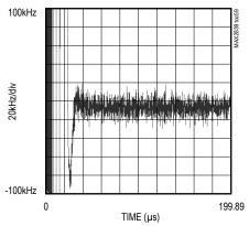
TX-TO-RX TURNAROUND FREQUENCY GLITCH SETTLING
