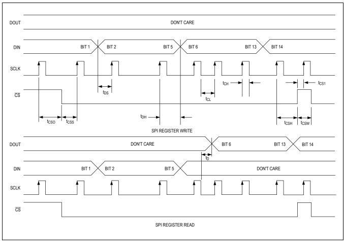
Figure 1. 4-Wire SPI Serial-Interface Timing Diagram
