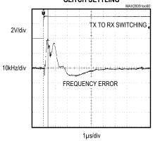
RX-TO-TX TURNAROUND FREQUENCY GLITCHING SETTLING
