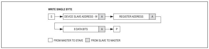
Figure 22. Write Byte Sequence
