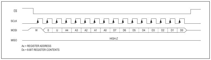
Figure 18. SPI Write Cycle
