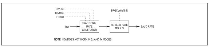
Figure 8. 2x and 4x Baud Rates
