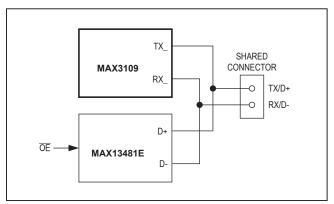
Figure 29. Connector Sharing with a USB Transceiver
