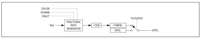
Figure 9. GPIO\_ Clock Pulse Generator
