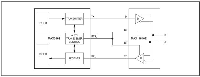
Figure 10. Auto Transceiver Direction Control
