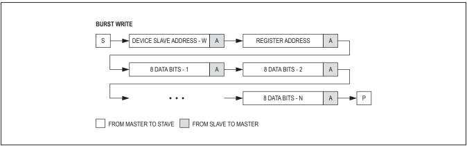
Figure 23. Burst Write Sequence
