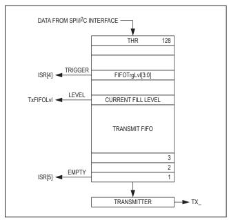
Figure 3. Transmit FIFO Signals
