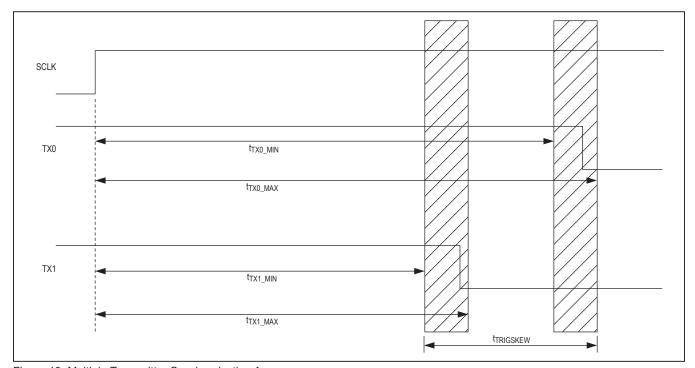
Figure 13. Multiple Transmitter Synchronization Accuracy
