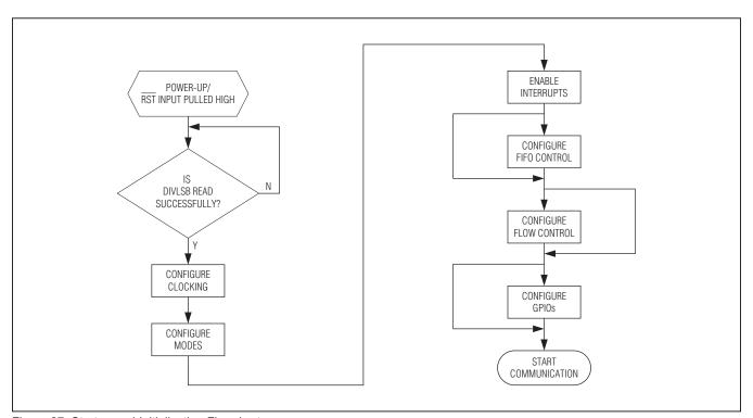
Figure 27. Startup and Initialization Flowchart
