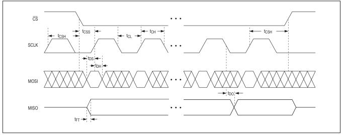
Figure 2. SPI Timing Diagram
