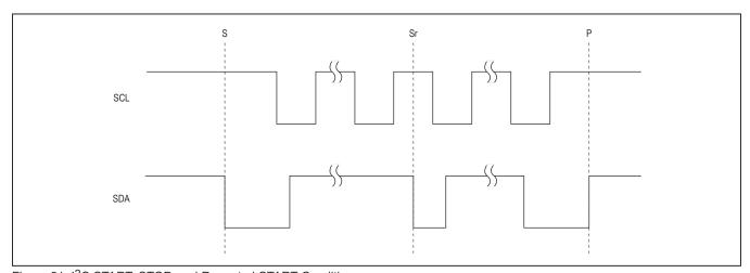
Figure 21. I<sup>2</sup>C START, STOP, and Repeated START Conditions
