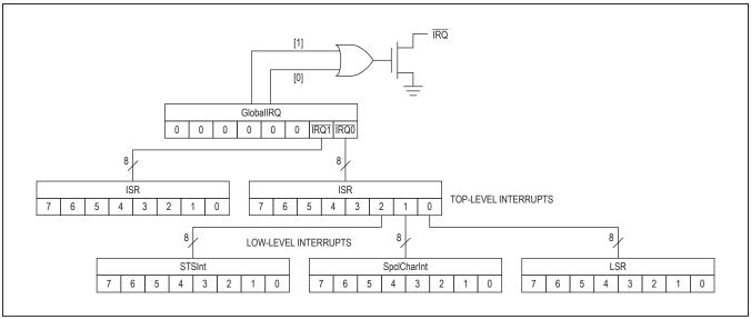
Figure 16. Simplified Interrupt Structure
