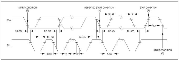
Figure 1. I<sup>2</sup>C Timing Diagram
