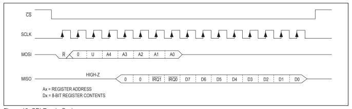
Figure 19. SPI Ready Cycle
