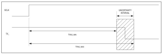
Figure 12. Single Transmitter Trigger Accuracy
