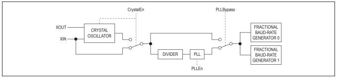
Figure 7. Clock Selection Diagram
