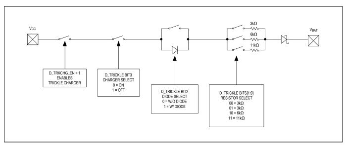
Figure 2. Trickle Charger Register (19h)
