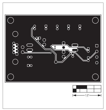
Figure 5. MAX3162 EV Kit PCB Layout—Solder Side
