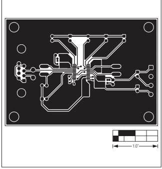
Figure 4. MAX3162 EV Kit PCB Layout—Component Side
