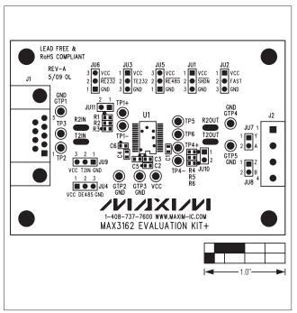
Figure 3. MAX3162 EV Kit Component Placement Guide
