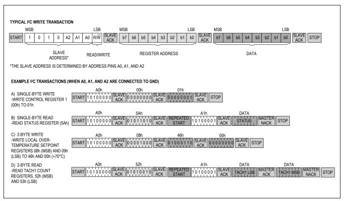
Figure 6. I<sup>2</sup>C Communication Examples
