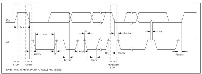
Figure 1. I<sup>2</sup>C Timing Diagram
