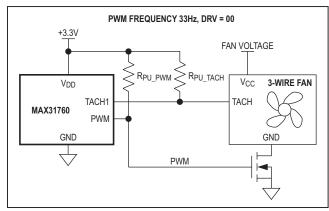
Figure 2b. PWM Supply Modulation (3-Wire Fan)
