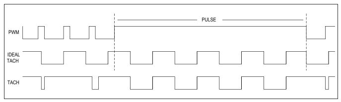
Figure 3. Pulse Stretching to Process TACH Information
