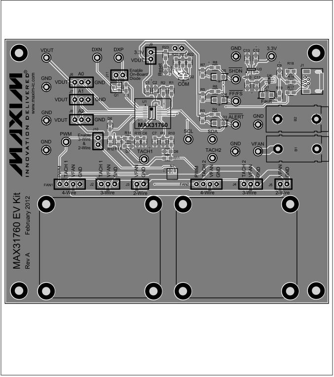
Figure 6. MAX31760 EV Kit PCB Layout—Top
