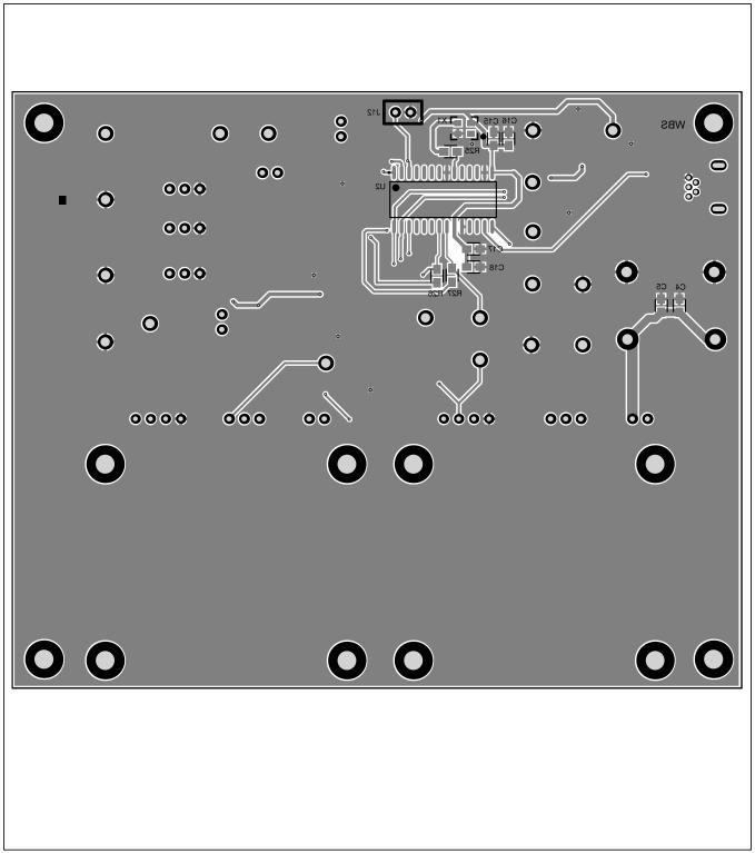
Figure 7. MAX31760 EV Kit PCB Layout—Bottom
