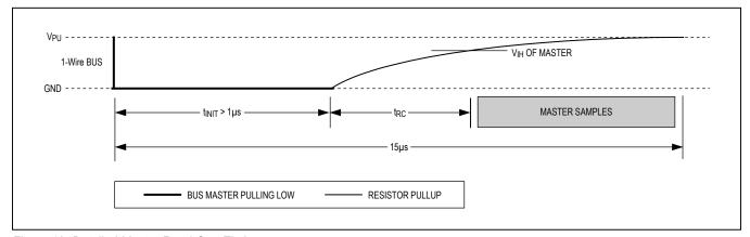
Figure 12. Detailed Master Read-One Timing
