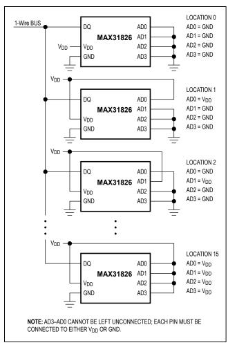
Figure 14. Address Programming Diagram—V<sub>DD</sub> Powered
