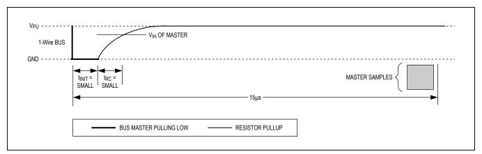
Figure 13. Recommended Master Read-One Timing
