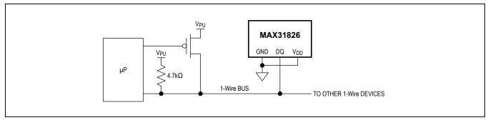
Figure 1. Supplying the Parasite-Powered MAX31826 During Temperature Conversions
