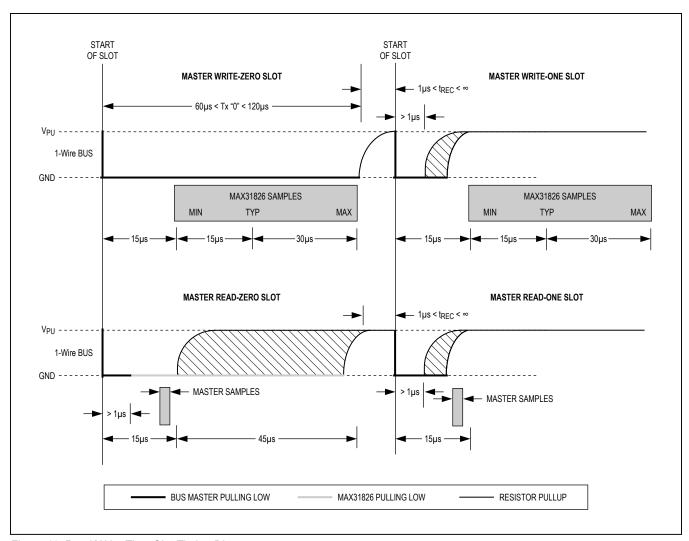
Figure 11. Read/Write Time Slot Timing Diagram
