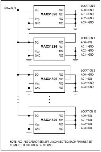
Figure 15. Address Programming Diagram—Parasite Powered
