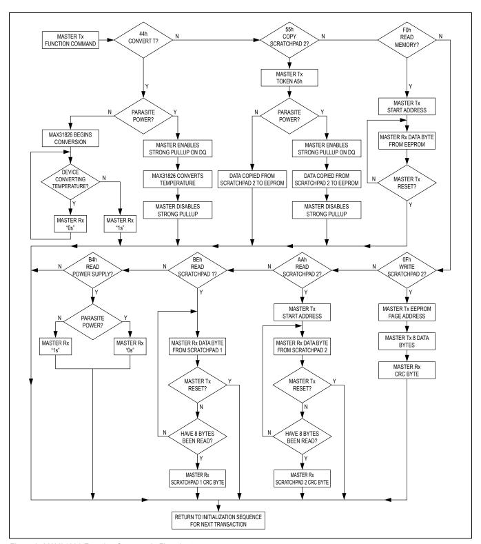
Figure 8. MAX31826 Function Commands Flowchart
