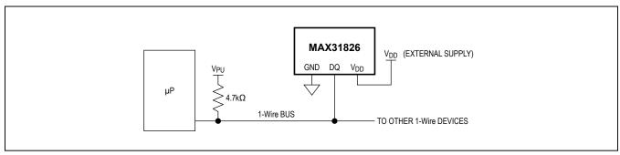
Figure 2. Powering the MAX31826 with an External Supply
