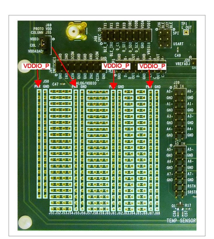
Figure 1. MAX32600 EV Kit Prototype Area
