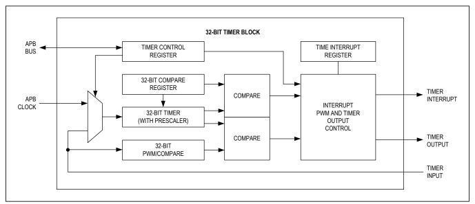
Figure 3. Timer Block Diagram, 32-Bit Mode
