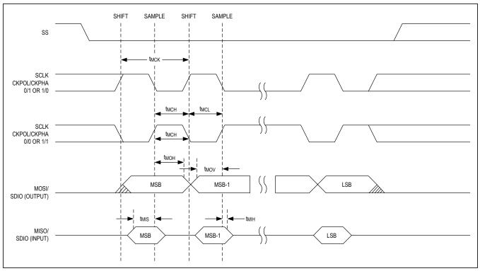
Figure 1. SPI Master and SPI XIP Master Timing
