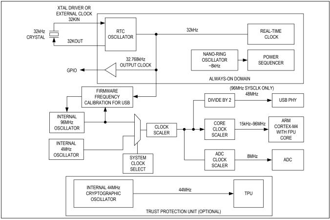
Figure 2. MAX32620/MAX32621 Clock Scheme (TPU on MAX32621 Only)
