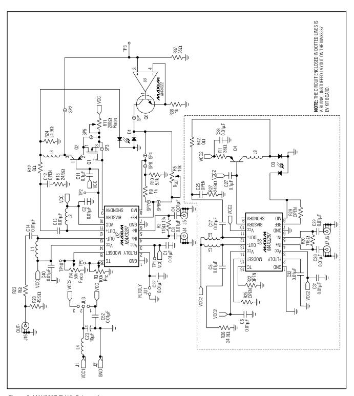
Figure 2. MAX3287 EV Kit Schematic
