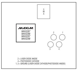
Figure 1. Optical Connection Diagram
