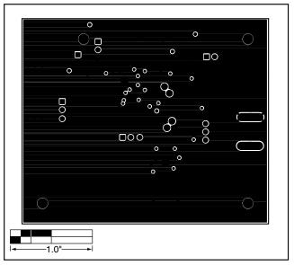
Figure 6. MAX3287 EV Kit PC Board Layout—Ground Plane
