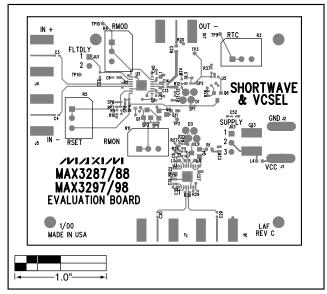
Figure 3. MAX3287 EV Kit Component Placement Guide
