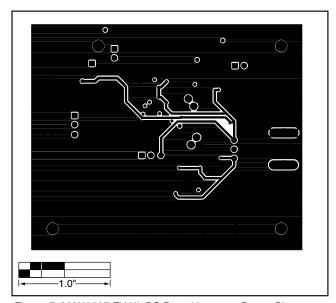
Figure 7. MAX3287 EV Kit PC Board Layout—Power Plane
