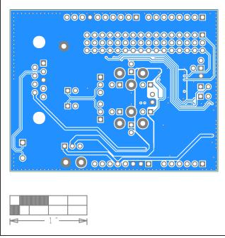
MAX33040E Shield PCB Layout—Bottom
