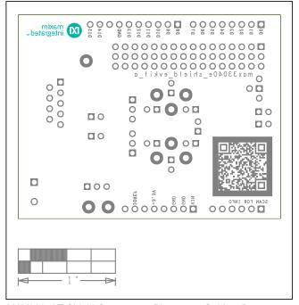
MAX33040E Shield Component Placement Guide—Bottom Silkscreen
