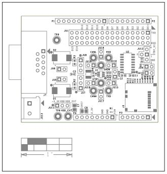
MAX33040E Shield Component Placement Guide—Top Silkscreen
