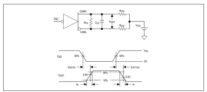
Figure 1. Transmitter Test Circuit and Timing Diagram
