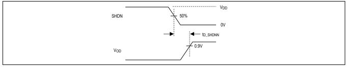
Figure 7. Shutdown Mode Timing Diagram
