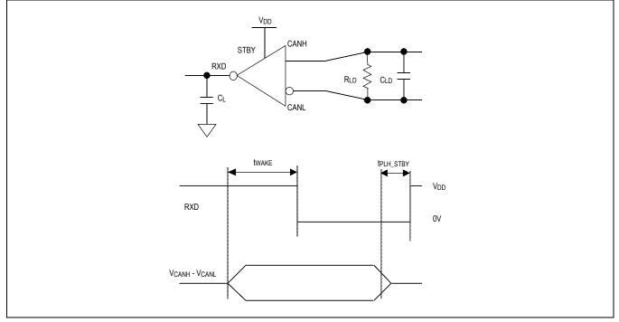
Figure 5. Standby Receiver Propagation Delay
