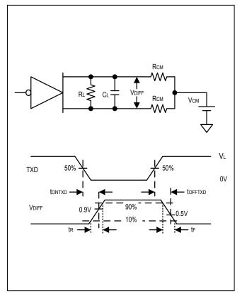
Figure 1. Transmitter Test Circuit and Timing Diagram
