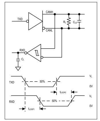
Figure 2. TXD to RXD Loop Delay
