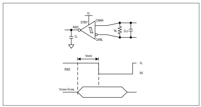
Figure 5. Standby Receiver Propagation Delay
