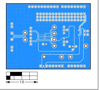
MAX33071E Shield EV Kit PCB Layout Diagram—Bottom View
