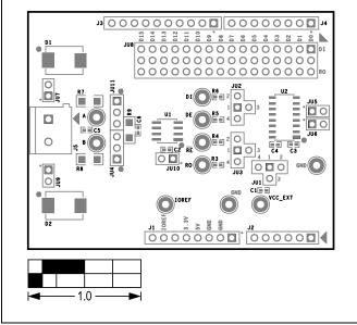
MAX33071E Shield EV Kit PCB Layout Diagram—Top Silkscreen
