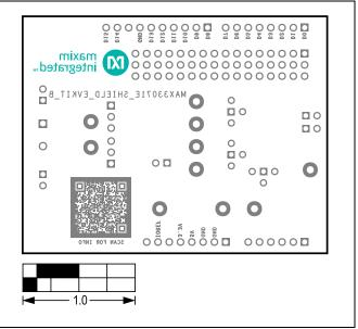
MAX33071E Shield EV Kit PCB Layout Diagram—Bottom Silkscreen
