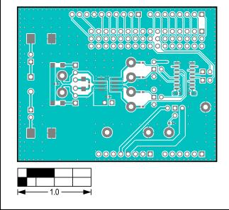
MAX33071E Shield EV Kit PCB Layout Diagram—Top View
