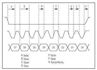
Figure 2. Serial-Interface Timing Diagram
