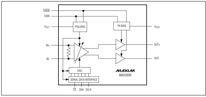
Figure 1. MAX3509 Functional Diagram
