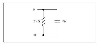
Figure 3. Typical Equivalent Input Circuit
