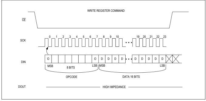
Figure 20. Write Register Opcode Command Protocol
