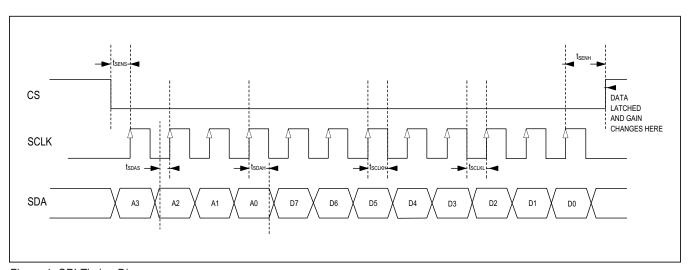
Figure 1: SPI Timing Diagram
