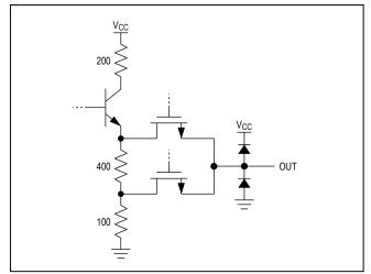
Figure 1. Equivalent Output Circuit
