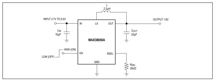
Figure 1. 1.8V Buck Converter Using the MAX38650A
