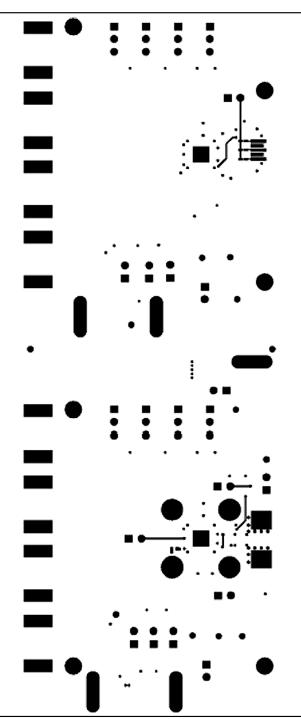
Figure 9. MAX3865 EV Kit PC Board Layout—Solder Side
