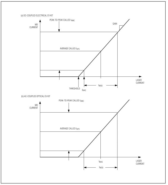
Figure 1. Relation Between Chip-Output Currents and Monitor-Diode Currents
