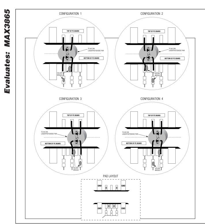
Figure 2. Attachment of a Laser Diode/Monitor Diode to the MAX3865 EV Kit
