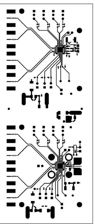
Figure 6. MAX3865 EV Kit PC Board Layout—Component Side
