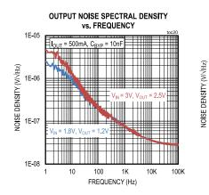
OUTPUT NOISE SPECTRAL DENSITY vs. FREQUENCY
