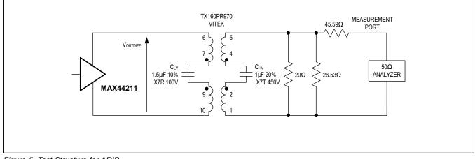
Figure 5. Test Structure for ARIB
