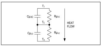
Figure 2. Thermal Flow Model
