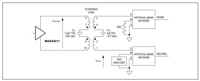
Figure 3. Test Structure for Cenelec
