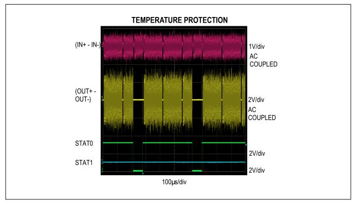
Figure 1. Temperature Protection
