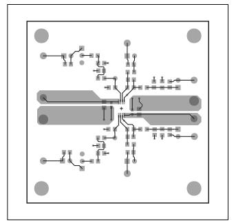
Figure 3. MAX44242 EV Kit PCB Layout—Component Side
