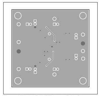
Figure 4. MAX44242 EV Kit PCB Layout—Solder Side
