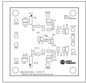
Figure 2. MAX44242 EV Kit Component Placement Guide—Component Side
