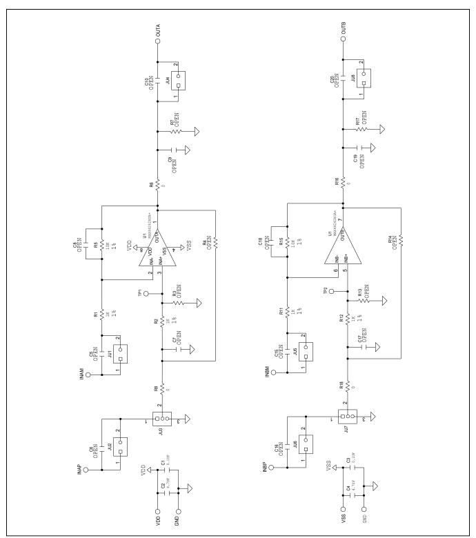
Figure 1. MAX44242 EV Kit Schematic
