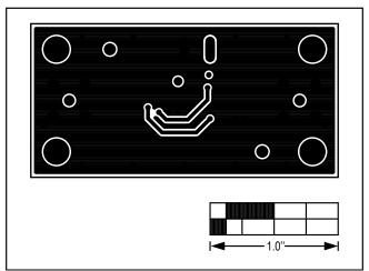
Figure 4. MAX442810 EV Kit PCB Layout—Solder Side
