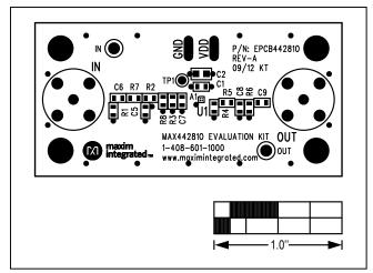
Figure 2. MAX44281O EV Kit Component Placement Guide—Component Side
