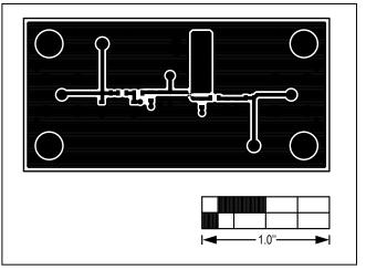
Figure 3. MAX44281O EV Kit PCB Layout—Component Side
