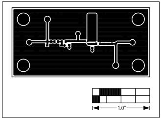
Figure 3. MAX44281U EV Kit PCB Layout—Component Side
