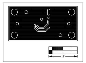
Figure 4. MAX44281U EV Kit PCB Layout—Solder Side
