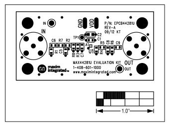
Figure 2. MAX44281U EV Kit Component Placement Guide—Component Side
