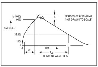
Figure 7. Human Body Model Current Waveform
