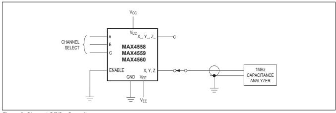
Figure 5. Channel Off/On-Capacitance
