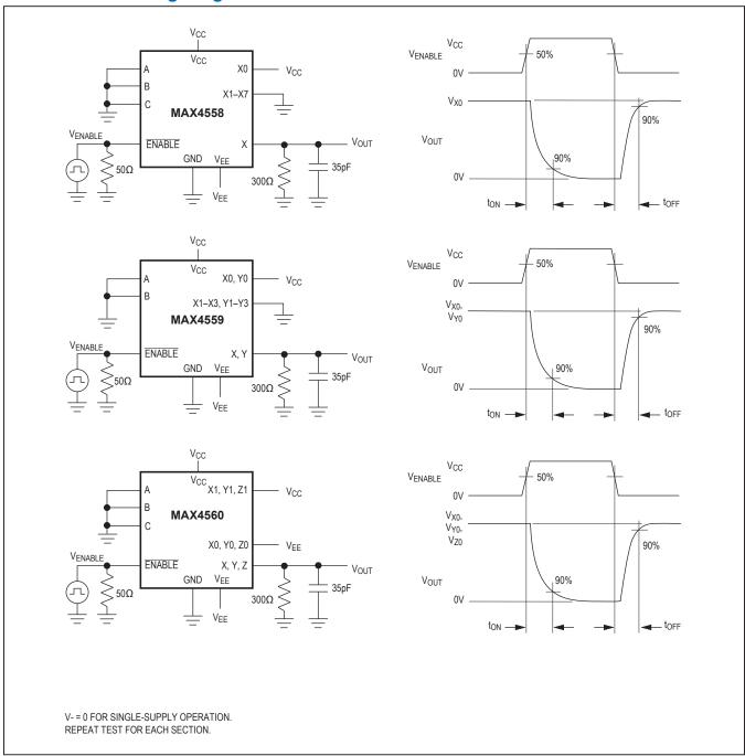
Figure 1. Switching Times
