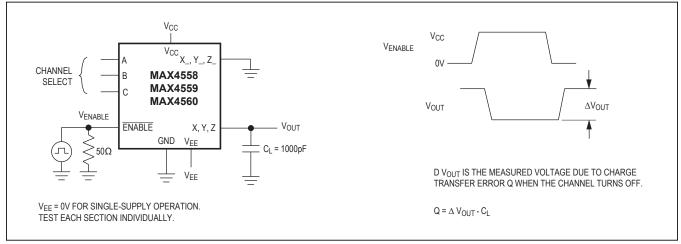
Figure 3. Charge Injection
