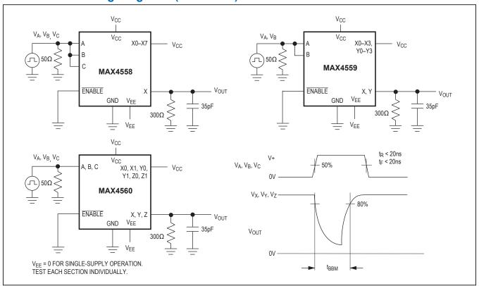
Figure 2. Break-Before-Make Interval
