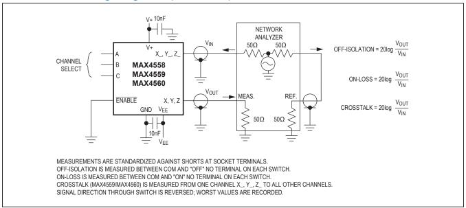
Figure 4. Off-Isolation/On-Channel Bandwidth and Crosstalk
