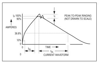
Figure 4. Human Body Current Waveform
