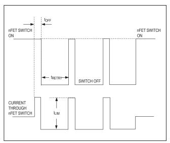
Figure 2. Autoretry Timing Diagram
