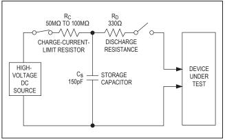
Figure 5. IEC 61000-4-2 ESD Test Model
