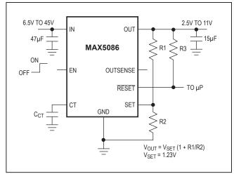
Figure 2. Setting the Adjustable Output Voltage
