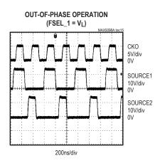
(See the *Typical Application Circuit*, unless otherwise noted.  $V+ = V_{IN\_HIGH} = 14V$ , unless otherwise noted.  $V+ = V_{IN\_HIGH}$  means that N1 is shorted externally.)
