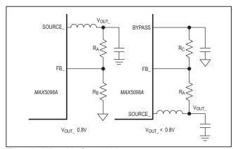
Figure 3. Adjustable Output Voltage
