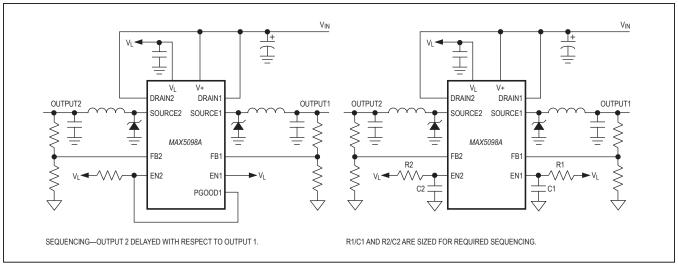
Figure 2. Power-Supply Sequencing Configurations
