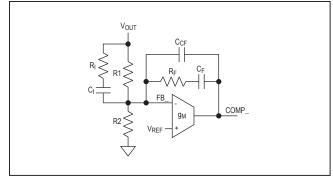
Figure 5. Type III Compensation Network
