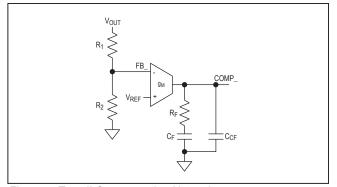
Figure 4. Type II Compensation Network
