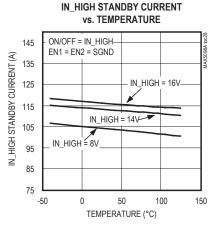
(See the *Typical Application Circuit*, unless otherwise noted. V+ = V<sub>IN\_HIGH</sub> = 14V, unless otherwise noted. V+ = V<sub>IN\_HIGH</sub> means that N1 is shorted externally.)
