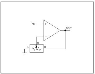
Figure 3. Variable Gain Noninverting Amplifier
