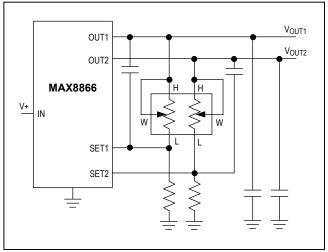
Figure 5. Adjustable Dual Linear Regulator
