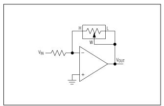
Figure 4. Variable Gain Inverting Amplifier
