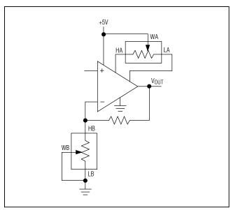
Figure 11. Offset Voltage Adjustment Circuit
