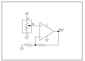
Figure 8. Positive LCD Bias Control Using a Voltage-Divide
