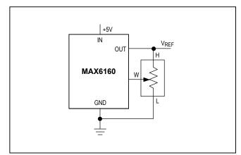
Figure 6. Adjustable Voltage Reference
