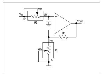
Figure 10. Programmable Filter
