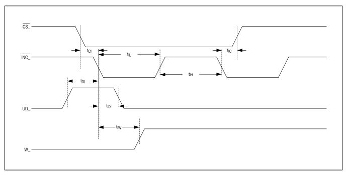
Figure 2. Up/Down Interface Timing Diagram
