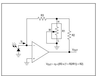
Figure 7. Variable Gain I-to-V Converter
