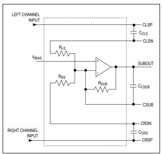
Figure 12. Subwoofer Output Stage
