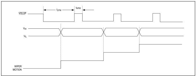
Figure 2b. Repetitive Input-Pulse Separation Time
