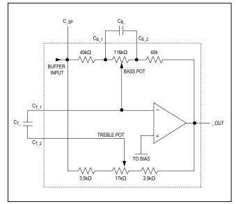
Figure 7. Bass/Treble Output Stage
