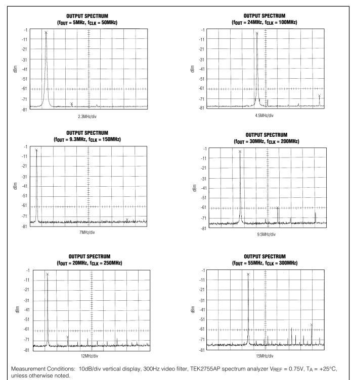
Figure 3. Spectrum Analyzer Plots
