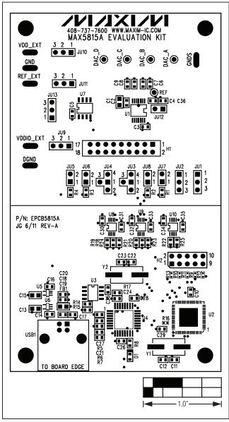
Figure 5. MAX5815A EV Kit Component Placement Guide— Component Side
