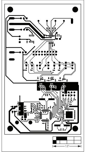
Figure 6. MAX5815A EV Kit PCB Layout—Component Side
