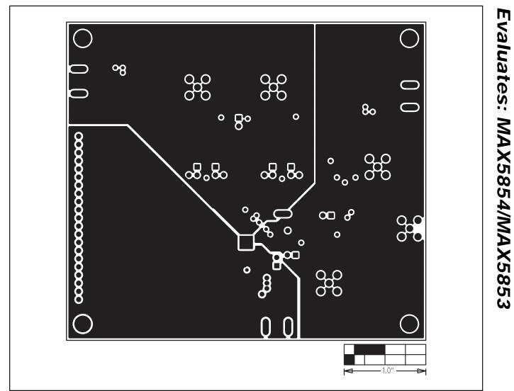
Figure 6. MAX5854 EV Kit PC Board Layout—Power Planes (Layer 3)
