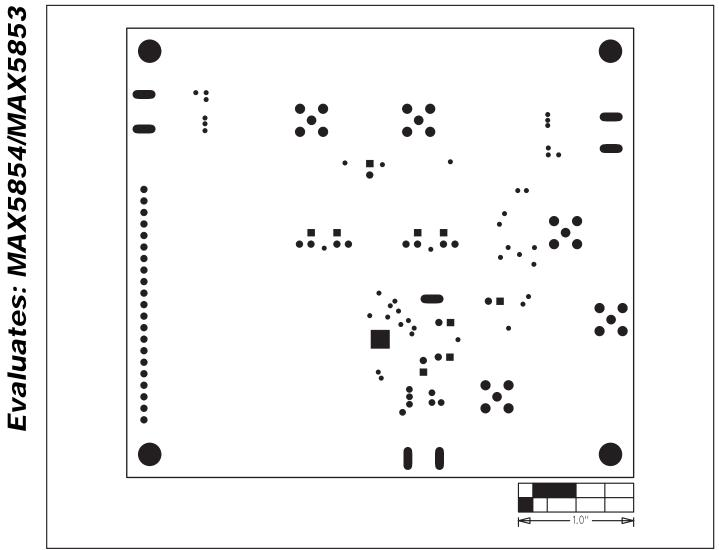
Figure 7. MAX5854 EV Kit PC Board Layout—Solder Side (Layer 4)
