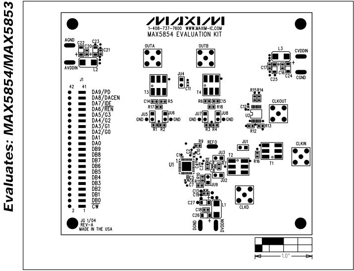
Figure 3. MAX5854 EV Kit Component Placement Guide—Component Side
