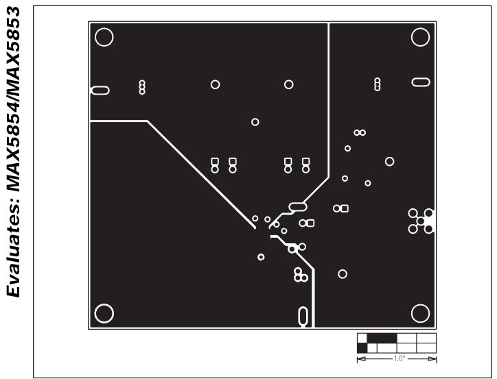
Figure 5. MAX5854 EV Kit PC Board Layout—Ground Planes (Layer 2)
