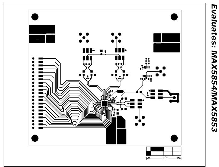
Figure 4. MAX5854 EV Kit PC Board Layout—Component Side (Layer 1)
