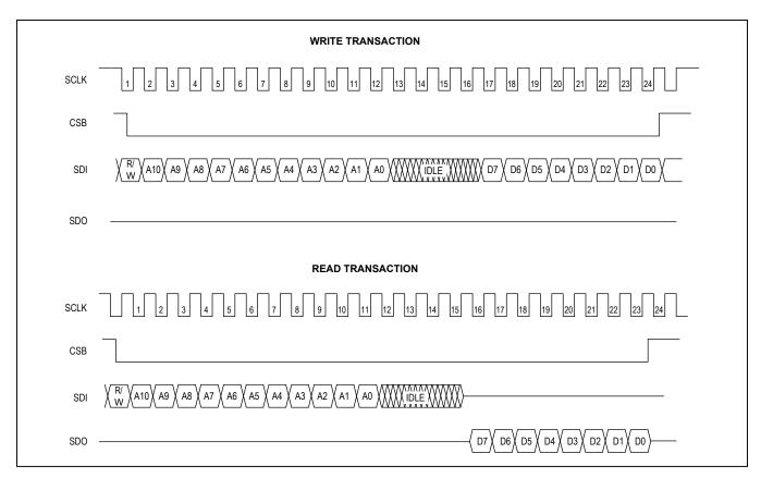
Figure 15. SPI Write and Read Transactions
