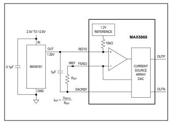
Figure 2. Reference Architecture, External Reference Configuration
