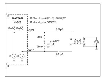
Figure 3. Typical DAC Output Configuration
