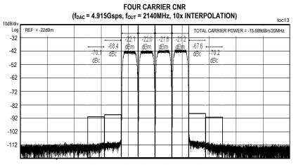
CENTER = 2140MHz, SPAN = 80MHz, RBW = 30kHz, VBW = 3kHz, SWEEP = 1.104s, ATTEN = 0dB
