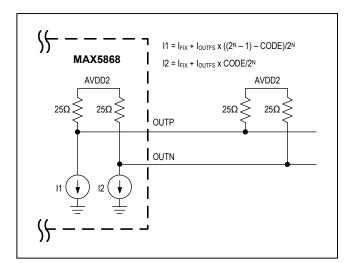
Figure 4. Output Configuration for Low-Frequency Operation
