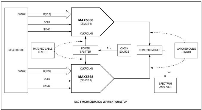
Figure 11. DAC Synchronization Verification Setup
