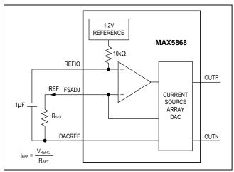
Figure 1. Reference Architecture, Internal Reference Configuration
