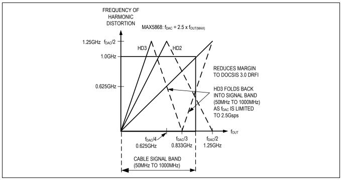
Figure 7. Example of Incorrect Frequency Planning
