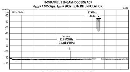
CENTER = 900MHz, SPAN = 1.2GHz, RBW = 30kHz, VBW = 3kHz. SWEEP = 13.4s. ATTEN = -6dB
