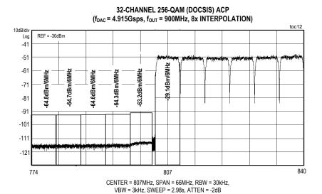
\*SETUP OPTIMIZED FOR NOISE FLOOR. GAIN FLATNESS IS IMPROVED BY INCREASING ATTENUATION.
