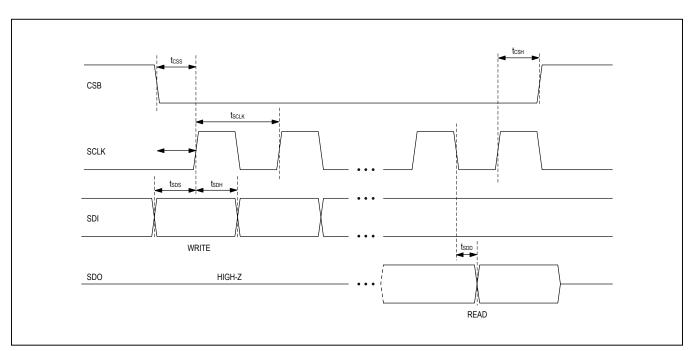
Figure 14. SPI Timing
