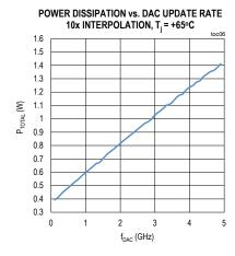
$(V_{AVDD} = V_{AVCLK} = V_{DD} = 1.0V, V_{AVDD2} = V_{AVCLK2} = V_{DD2} = 1.8V, P_{CLK} = 0dBm, 16-bit word mode, I_{OUTFS} = 29.5385mA, output is <math>50\Omega$  double-terminated and transformer coupled, external reference at 1.20V,  $R_{SET} = 1.3k\Omega$  between FSADJ and DACREF,  $T_A = +25^{\circ}C$ ,  $T_J = +65^{\circ}C$ , unless otherwise noted.)
