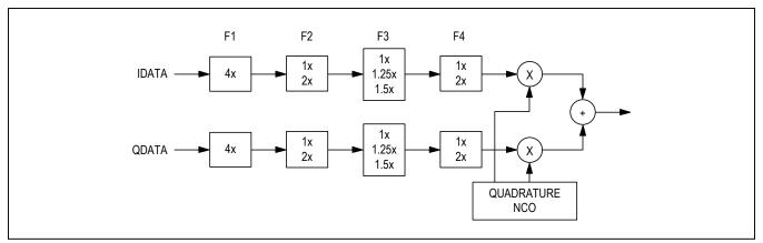
Figure 6. Interpolator/Modulator Block Diagram
