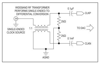
Figure 4. Differential Clock-Signal GenerationAnalog Output
