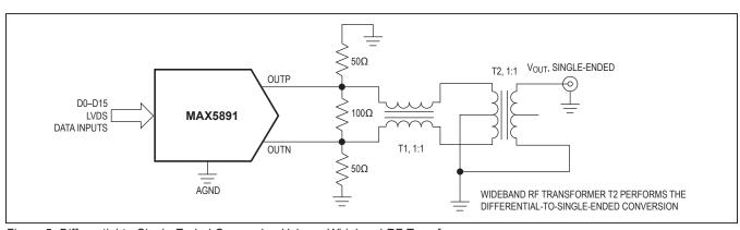
Figure 5. Differential-to-Single-Ended Conversion Using a Wideband RF Transformer
