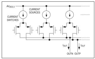
Figure 2. Simplified Analog Output Structure
