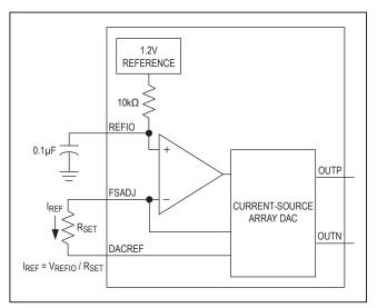
Figure 1. Reference Architecture, Internal Reference Configuration
