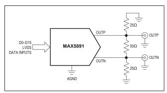
Figure 6. Differential Output Configuration
