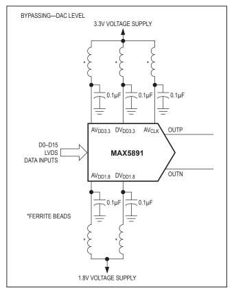
Figure 7. Recommended Power-Supply Decoupling and Bypassing Circuitry
