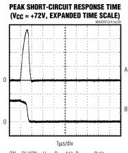
$0N = RLY0N = V_{DD}, \ R_L = 1\Omega, \ R_{RTIM} = 2k\Omega$ A: I<sub>OUT</sub>, 5A/div B: V<sub>GATE</sub>, 50V/div
