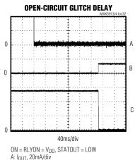
A: I<sub>OUT</sub>, 20mA/div B: V<sub>STAT</sub>, 5V/div C: VGATE, 20V/div
