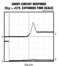
$\begin{array}{l} 0N = RLYON = V_{DD}, \, R_L = 1\Omega, \, R_{RTIM} = 2k\Omega \\ A: \, I_{OUT}, \, 200mA/div \\ B: \, V_{GATE}, \, 20V/div \end{array}$
