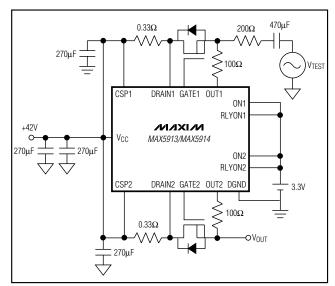
Figure 4. Channel-to-Channel Crosstalk Test Circuit
