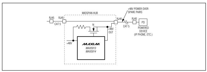
Figure 10. Power Sent Over Spare Pairs
