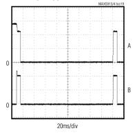
$RTRYEN = V_{DD}$ ,  $RLYON = ON = V_{DD}$ , DC = 4%,  $R_{RTIM}=2k\Omega,~R_L=100\Omega$ A: VGATE, 20V/div
