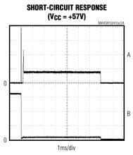
ON = RLYON = V<sub>DD</sub> A: I<sub>OUT</sub>, 200mA/div B: V<sub>GATE</sub>, 20V/div
