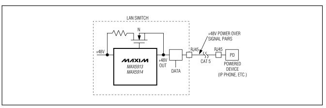
Figure 9. Power Sent Over Signal Pairs
