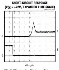
$0N = RLYON = V_{DD}, \ R_L = 1\Omega, \ R_{RTIM} = 2k\Omega$ A: I<sub>OUT</sub>, 200mA/div B: V<sub>GATE</sub>, 50V/div
