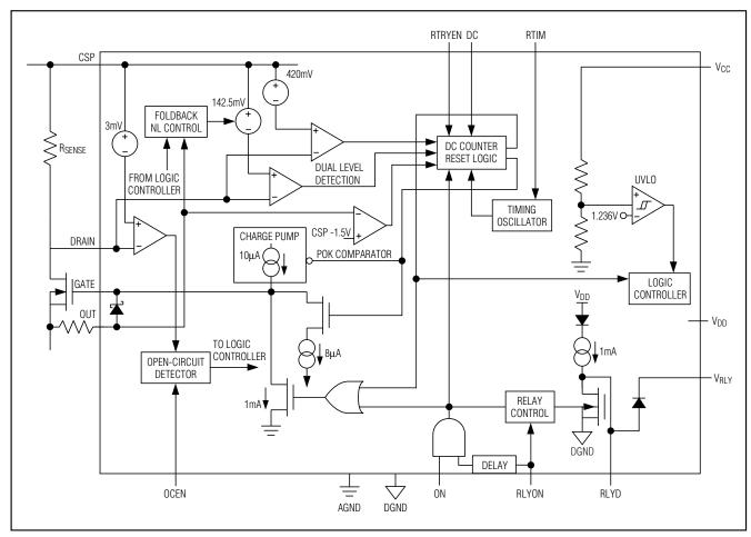
Figure 6. Functional Diagram
