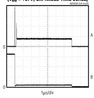
$ON = RLYON = V_{DD}, R_L = 1\Omega, R_{RTIM} = 2k\Omega$  A:  $I_{OUT}$ , 5A/div B:  $V_{GATE}$ , 20V/div
