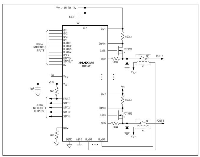
Figure 5. Typical Application Circuit
