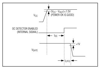
Figure 2. Open-Circuit Detector Deglitch Delay
