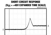
$0N=RLY0N=V_{DD},\,R_L=1\Omega,\,R_{RTIM}=2k\Omega$  A:  $I_{OUT},\,200mA/div$  B:  $V_{GATE},\,20V/div$
