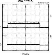
ON = RLYON = V<sub>DD</sub> A: I<sub>OUT</sub>, 200mA/div B: V<sub>GATE</sub>, 50V/div
