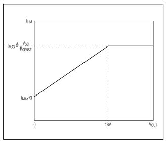
Figure 8. Foldback Current-Limit Response
