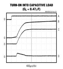
$$\begin{split} RLYON &= V_{DD} \\ A: V_{ON}, 5V/div \\ B: V_{GATE}, 20V/div \\ C: V_{OUT}, 20V/div \\ D: I_{OUT}, 100mA/div \end{split}$$
