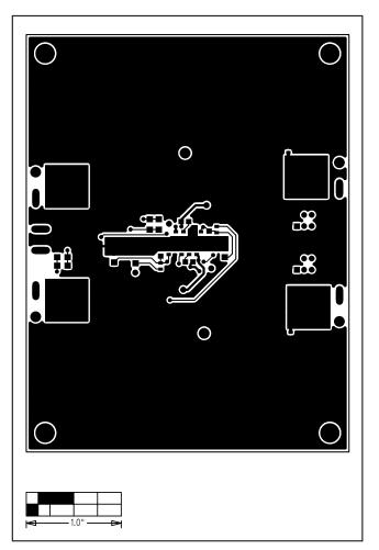
Figure 4. MAX5944 EV Kit PC Board Layout—Solder Side
