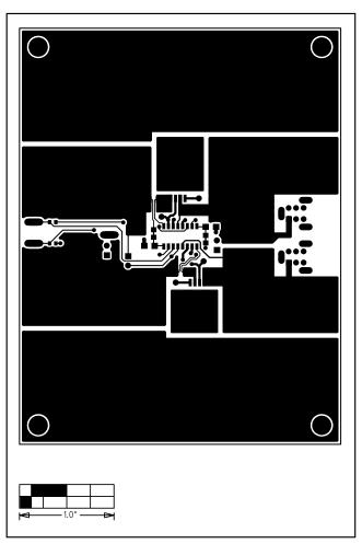
Figure 3. MAX5944 EV Kit PC Board Layout—Component Side
