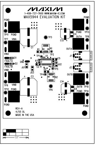
Figure 2. MAX5944 EV Kit Component Placement Guide— Component Side
