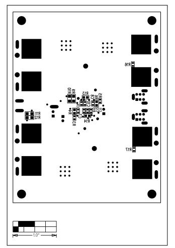
Figure 5. MAX5944 EV Kit Component Placement Guide— Solder Side
