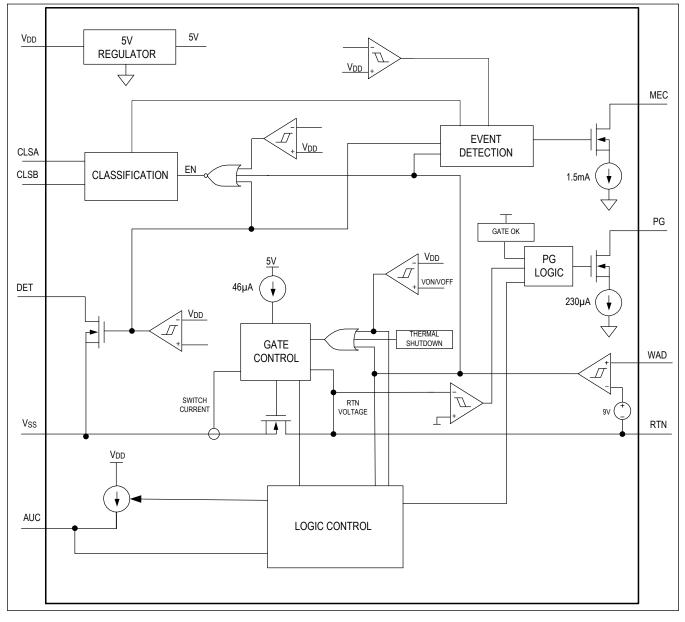
IEEE 802.3bt-Compliant, Powered Device Interface Controllers with Integrated 91W High-Power MOSFET
