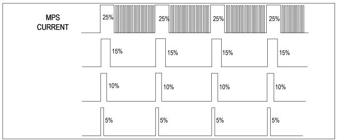
Figure 6. MPS Current with Different AUC Configuration
