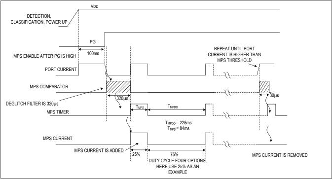
Figure 3. Intelligent MPS Behavior
