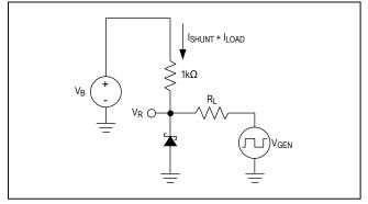
Figure 1. Load-Transient Circuit
