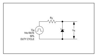
Figure 2. Startup Characteristics Test Circuit
