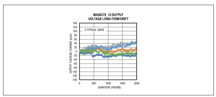
Figure 4. Output Voltage Long-Term Drift of the MAX6279 in Ceramic LCC Package
