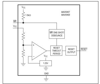
Figure 2. Functional Diagram
