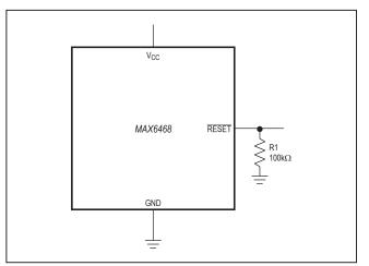
Figure 3.  $\overline{RESET}$  Valid to  $V_{CC} = 0V$
