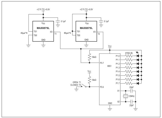
Figure 2. Interfacing Multiple Devices with a Microcontroller
