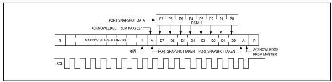
Figure 8. Reading Group B Ports of MAX7327
