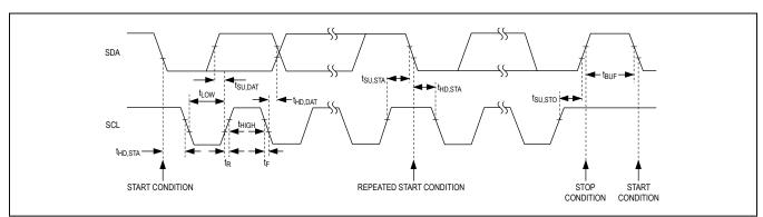
Figure 1. 2-Wire Serial Interface Timing Details
