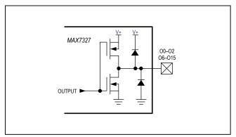
Figure 10. MAX7327 Push-Pull Output Port Structure
