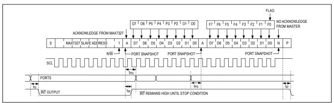
Figure 7. Reading Group A Ports of the MAX7327 (2 Data Bytes)
