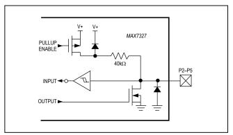
Figure 11. MAX7327 Open-Drain I/O Port Structure
