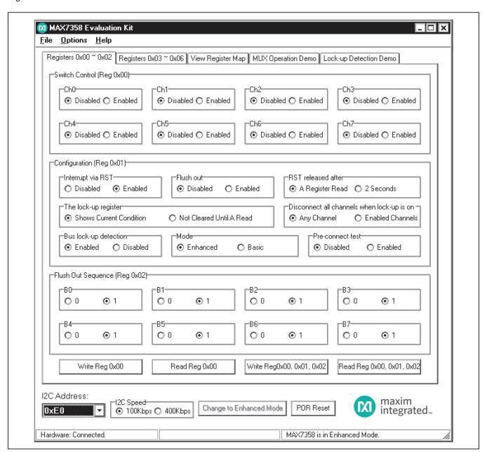
Figure 1. Software Main Window (Registers 0x00 ~ 0x02 Tab)
