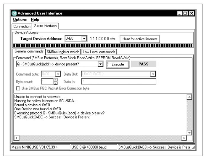
Figure 2. Advanced User Interface Window (2-Wire Interface Tab)
