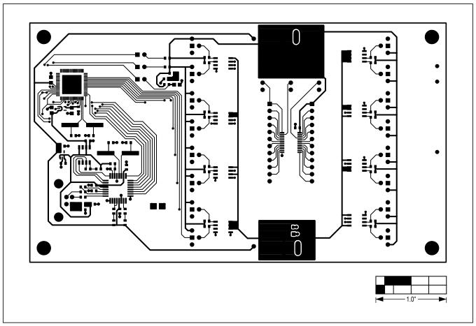
Figure 5. MAX7358 EV Kit PCB Layout—Component Side
