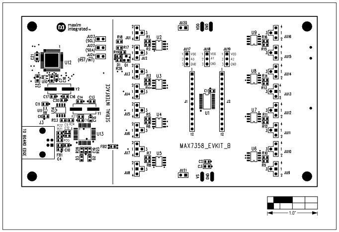
Figure 4. MAX7358 EV Kit Component Placement Guide—Component Side
