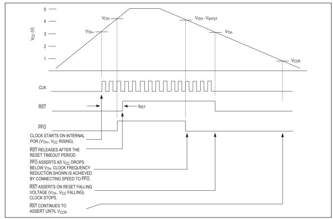
Figure 1. RST/RST and PFO Behavior During Power-Up and Brownout
