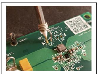
Figure 4. Example of Probing Sensitive Node
