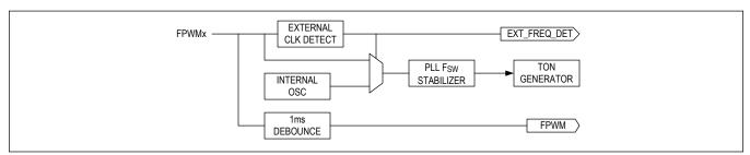
Figure 4. Frequency Tracking
