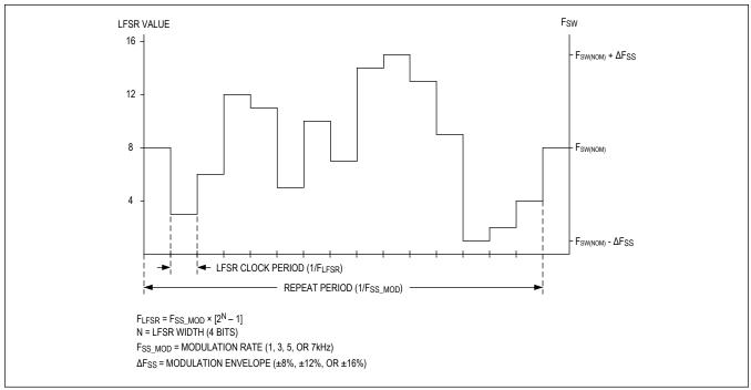
Figure 6. 4-Bit Pseudo-Random Modulation Signal Example
