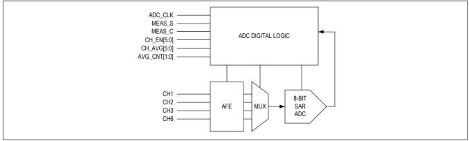
Figure 10. ADC Block Diagram
