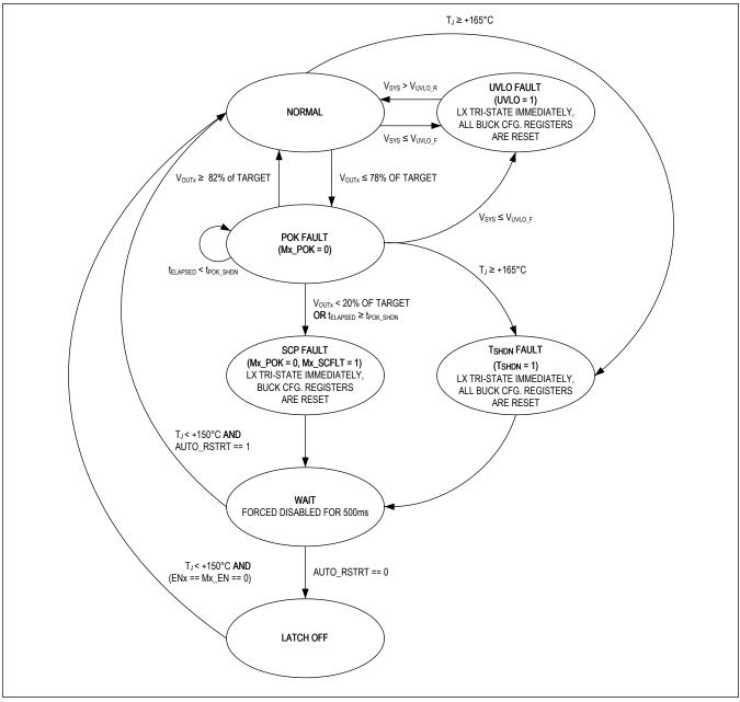
Figure 9. Fault Protection State Diagram
