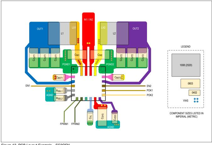
Figure 12. PCB Layout Example—FC2QFN
