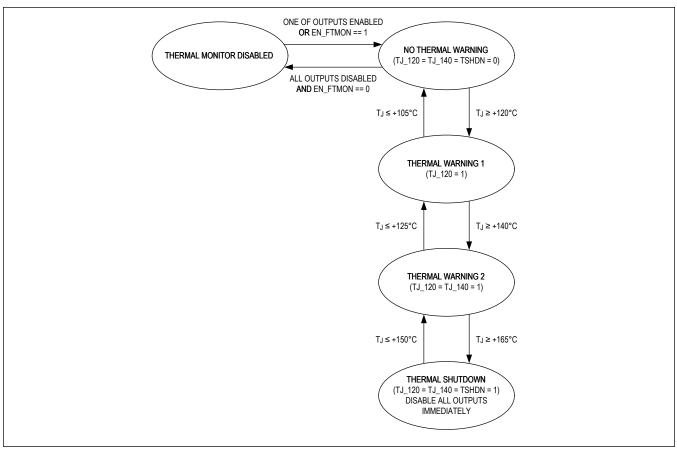
Figure 1. Thermal Warnings and Thermal Shutdown
