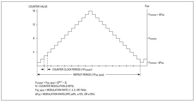
Figure 8. 4-Bit Triangular Modulation Signal Example
