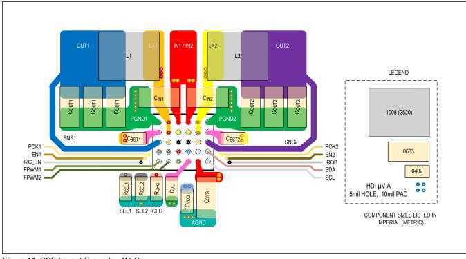
Figure 11. PCB Layout Example—WLP
