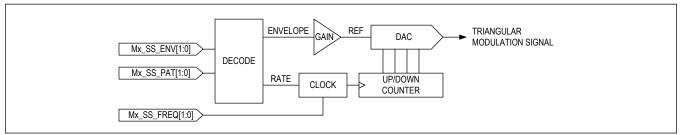
Figure 7. Triangular Modulator Engine
