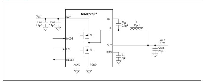
Figure 1. MAX77597ETBB+, Fixed Output Voltage (3.3V), 10-Pin TDFN
