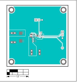
MAX77597 EV Kit PCB Layout Diagram—Top View
