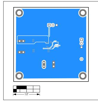
MAX77597 EV Kit PCB Layout Diagram—Bottom View
